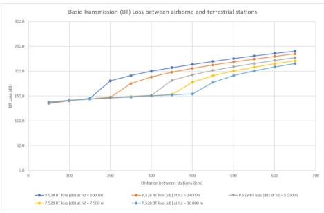
Figure 8.2-2 below shows how basic transmission loss change with altitude at particular distances between stations.
